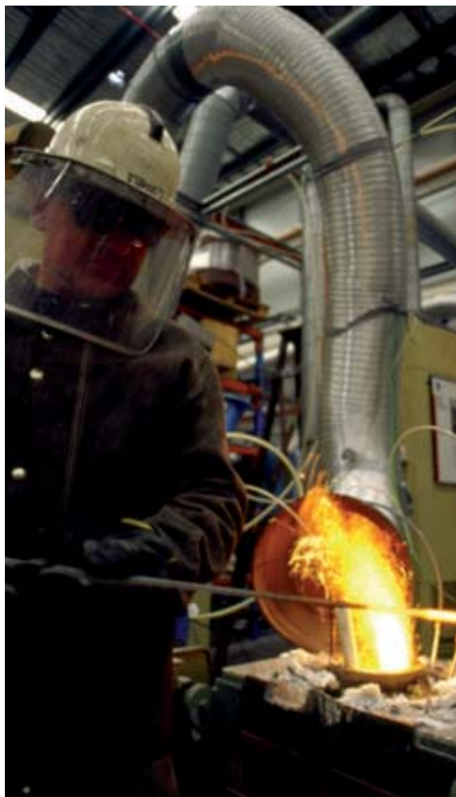
Sampling a molten bath during injection of charcoal at CSIRO Photo by C Pearson – mishey
