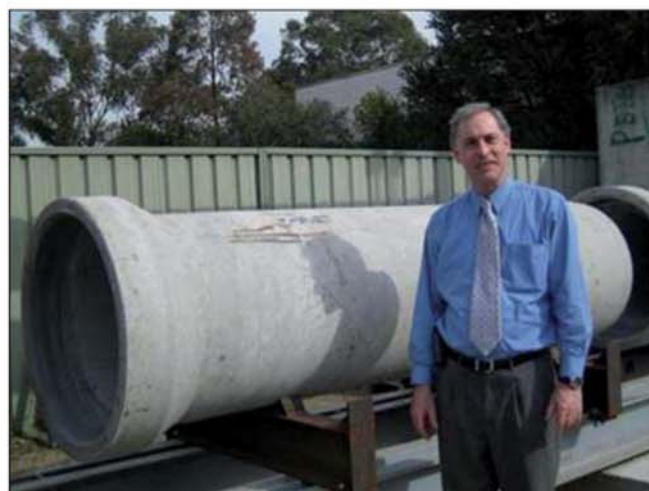
Figure 4 Geopolymer sewer pipe made from fly ash (photo courtesy of Rocla).
