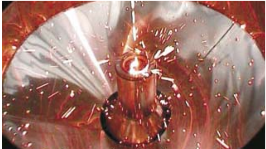
CSIRO'S DRY GRANULATION PROCESS: MOLTEN SLAG POURS ON TO A ROTARY DISC.
