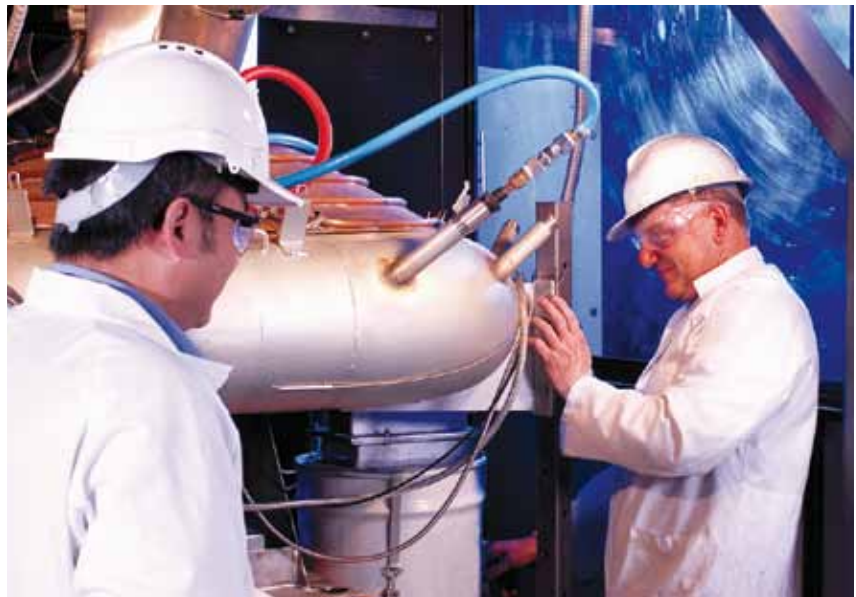
Dr Dongsheng Xie (left) and Bernie Washington inspecting the laboratory scale plant for integrated dry granulation and heat recovery process. PHOTO: MARK FERGUS
