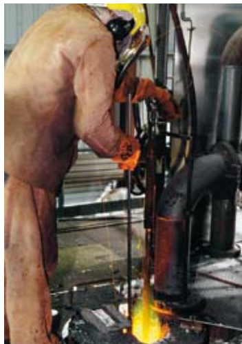
Terry Hall sampling molten slag from the SIROSMELT vessel.
