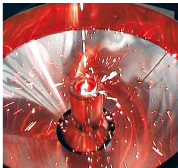
CSIRO's dry granulation process: molten slag pours on to a rotary disc. PHOTO: STEVE SANETSIS
