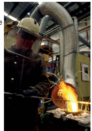
Sampling a molten iron bath during injection of charcoal (Photo by C Pearson)
